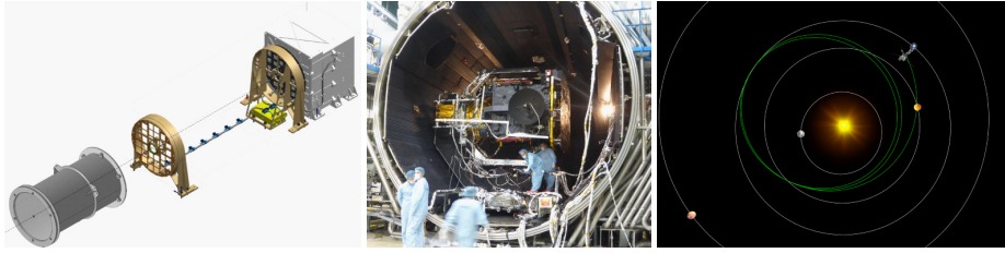
Fig. 1. Left: STIX images X-ray sources using moiré patterns produced by two tungsten grids placed in front of a sensor. Center: Solar Orbiter being prepared for launch. Right: Solar Orbiter completed its second Venus flyby maneuver November 2021.
