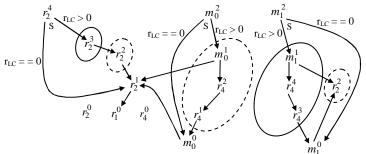
$r_2^2$  is drawn as two separate nodes for clarity (i.e., those two nodes are the same node). S: Annotation for the select operator (address annotations are not shown). Nodes generated within the loop are encircled (dotted: first pass, solid: second pass).
