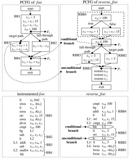
The PowerPC 860 instructions "stwu" and "lwzu" are used as push-like and pop-like instructions with r<sub>9</sub> being used as a memory pointer for state saving
