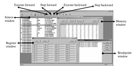
Figure 22: The GUI of the debugger tool.
