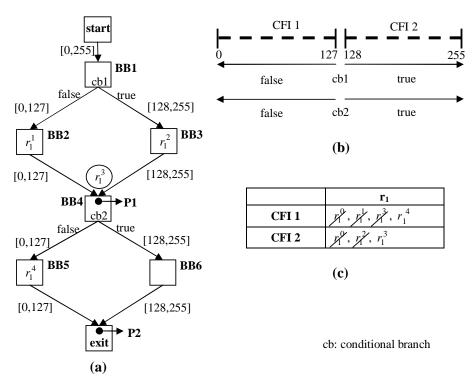
Figure 17: (a) A simple PCFG. (b) Corresponding CFIs. (c) Corresponding renaming table.
