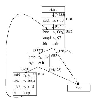
Figure 13: An example PCFG with labeled edges.
