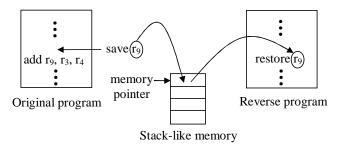
Figure 4: A diagram which illustrates the state saving method of the RCG algorithm.
