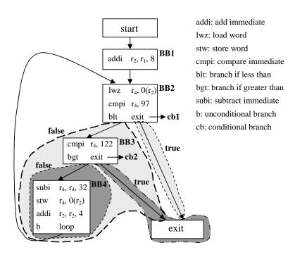
Figure 12: An example PCFG that shows the control flow regions.
