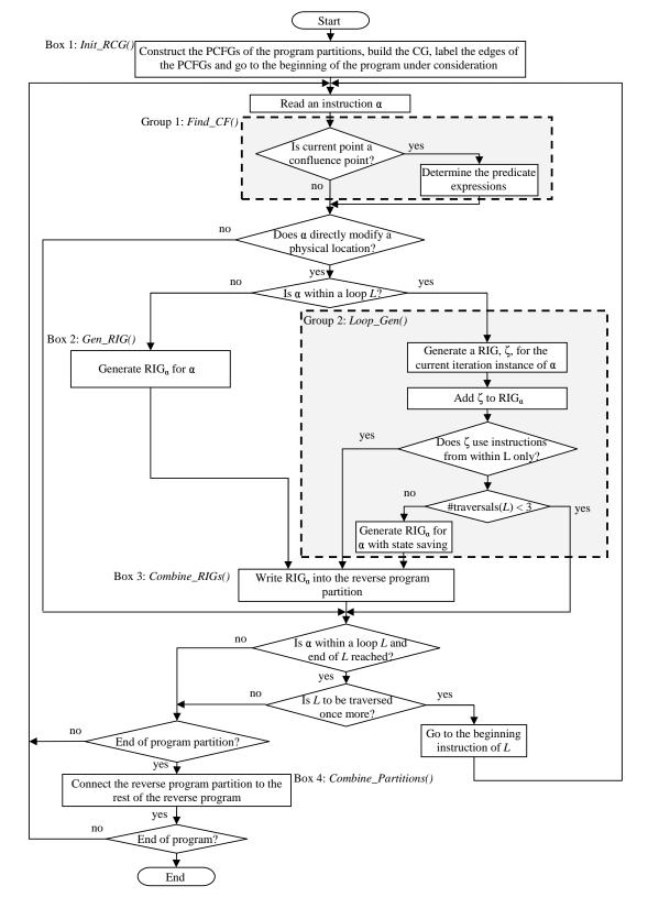
Figure 11: A high-level flowchart of the RCG algorithm.
