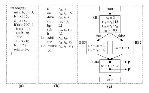
Figure 1: (a) A simple program in C. (b) Corresponding assembly instructions. (c) Corresponding PCFG.
