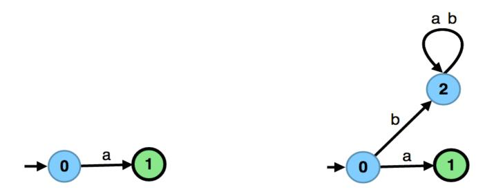
Undefined transitions are equivalent to transition into a sink state (from which one cannot recover)
