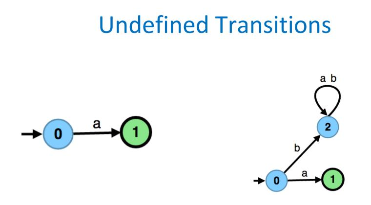
Undefined transitions lead to a sink state from where no input can be accepted
