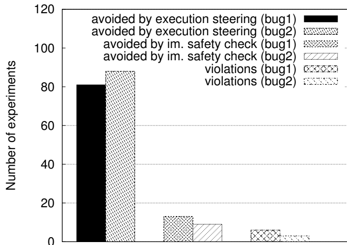
Fig. 17. In this experiment we run Paxos across an emulated wide area network using ModelNet. The experiment contains 200 runs in which the same two errors as in Figure 16 were injected. CrystalBall successfully avoided the inconsistencies in all but 6 and 3 cases, respectively.
